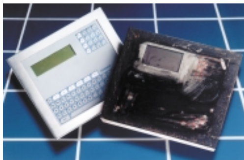
The above illustrates both a new and a badly fire-damaged but still fully functional T31.
